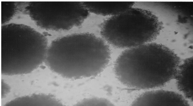
Figure 4. Large pellets with compacted morphological structure
